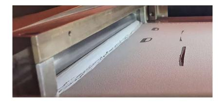
Excess melt energy causing clumping and sticking of powder around melt pool perimeters. This can potentially cause collisions with the roller and eventually part and build failure.
