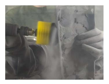
For optimal part performance, part cake firmness will be higher than for polyamide materials. Powder clumps should break apart and crumble with force. Use of a nylon bristle brush, particularly on a spinning tool, should remove the part cake easily.
